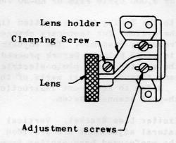
These adjustments are more readily made if the photo-electric cell is removed and a piece of transparent paper substituted. A still more convenient method is to remove the glass envelope and cathode from an old photo-electric cell, and substitute a transparent paper cathode attached to the cathode support wires. With either of these methods the spot can be accurately centered and adjusted for size.
