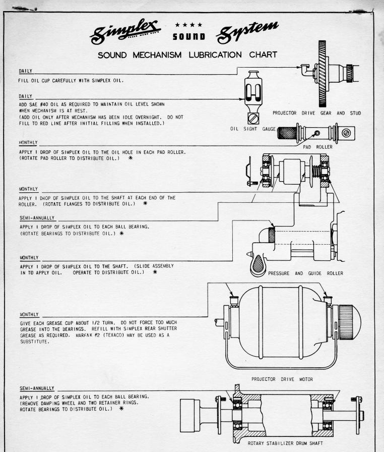
\* APPLY SIMPLEX OIL WITH A TOOTHPICK OR PIPE CLEANER. DO NOT OVER-LUBRICATE.
