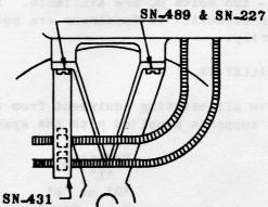
E. Take-up Belt. Adjust length as required and assemble. The take-up is driven from the sound mechanism.
